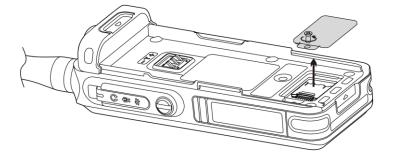
2. Install the TF card, put the card slot cover back in place, and then tighten the screw.
