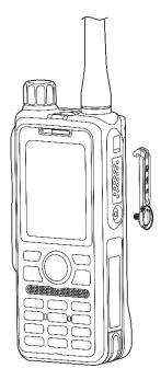
2. Insert the audio accessory plug into the accessory connector.
